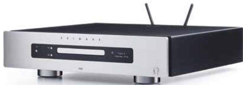
**CD35 Prisma** CD player combines a state-of-the-art TEAC dedicated CD drive, all-new reference balanced DAC stage feeding a finely tuned balanced analog output stage (with selectable fixed or variable output), and Prisma connectivity and control technology to create a complete digital music source. Each component part of the CD35 Prisma – the drive, the DAC, the output stage, and Prisma technology – contributes to what is simply the best CD player Primare has ever offered.
